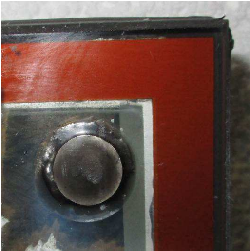
Fig. 3 Photo of the evacuation port (created by the ift).
